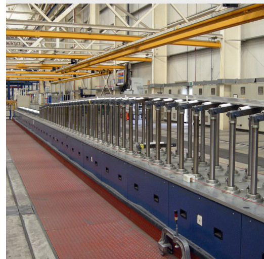
Computer controlled Wing Stringer Contour Forming machinery
